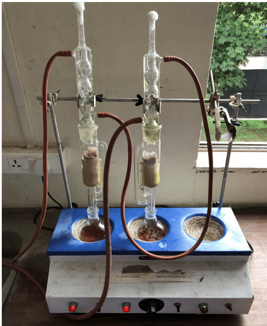
FIGURE 1: The Soxhlet apparatus used for preparing ginger extracts at the Department of Pharmacology, KIMS, KVV, Karad
