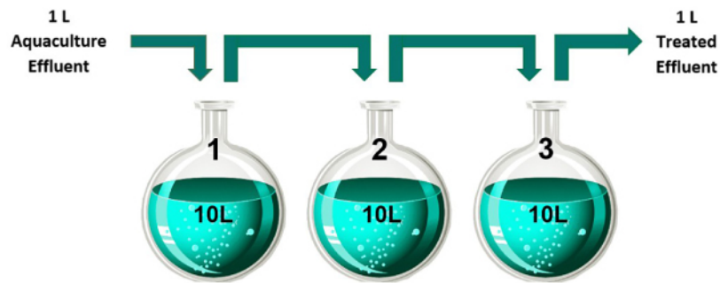
Figure 1. Schematic diagram of a semi-continuous cascade system, with three reactors of 10 L (addition and transfers of 1 L every 48 h).
