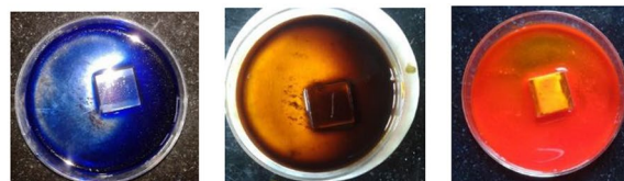
(b) dipped the coated electrodes in dyes [(i)methylene blue, (ii)extract of butea mono sperma flower, (iii)methyl orange]
