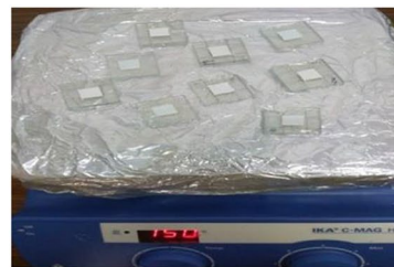
(a) Pasting of \text{TiO}_2/\text{ZnO} on FTO glass
