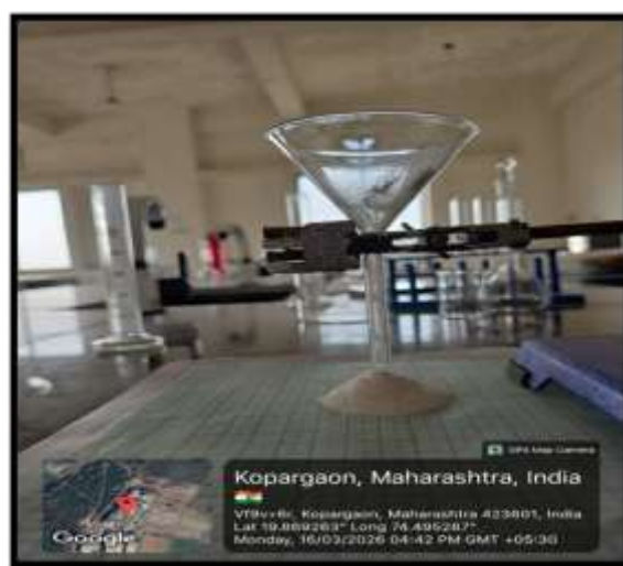
Fig. No. 08 Angle of Repose
