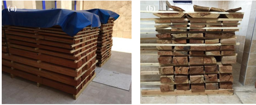
Figure 2. Covered open-air stack (a) and naturally ventilated indoor stack (b)
