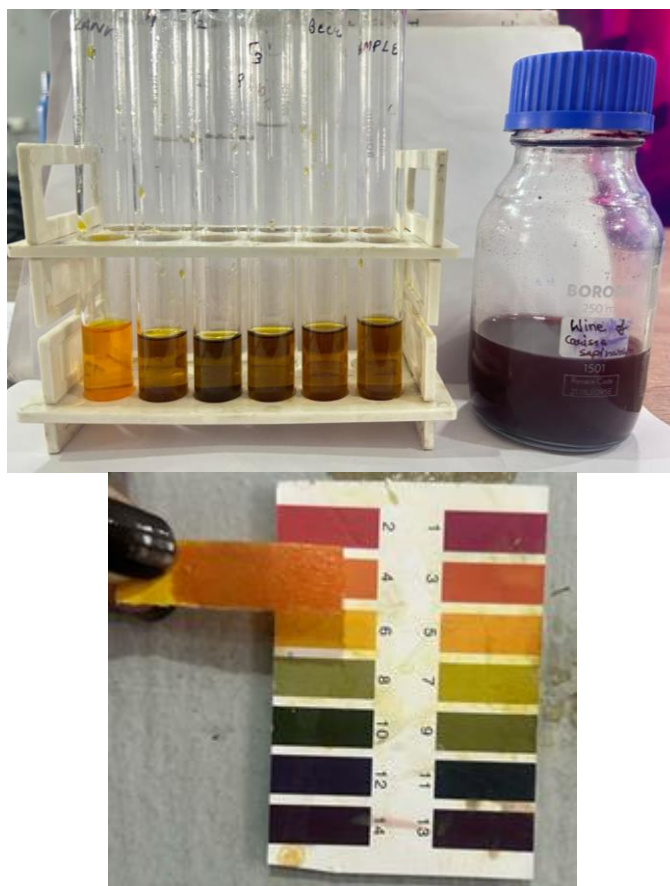
Figure 2 Test tubes containing dichromate acid and ethanol showing colour change due to the oxidation reaction between alcohol and dichromate ions
