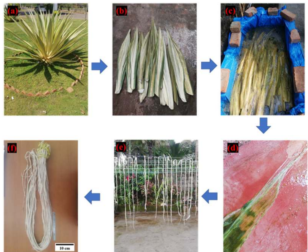
Figure 1. Furcraea foetida fiber extraction process (a) FF plant; (b) FF plant leaves; (c) water retting process; (d) separation of decayed substance; (e) drying of FF fiber; (f) extracted FF fiber bundles.
