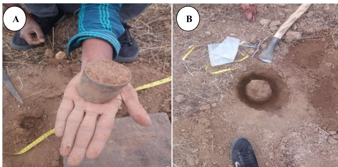
Figure 3. Soil sample collection at the field of the study area, (a) core sampler for bulk density and moisture contents determination; (b) Collection of composite soil samples from agricultural plots.
