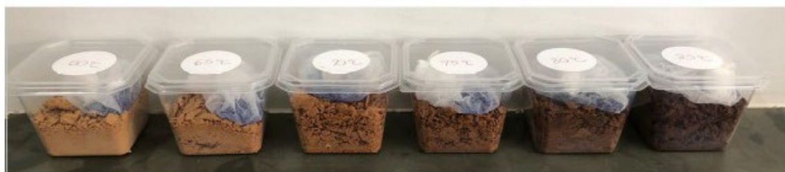
Figure 3. Tamarind pulps dried on a foam bed at temperatures of 60 °C, 65 °C, 70 °C, 75 °C, 80 °C, and 85 °C, from left to right.
