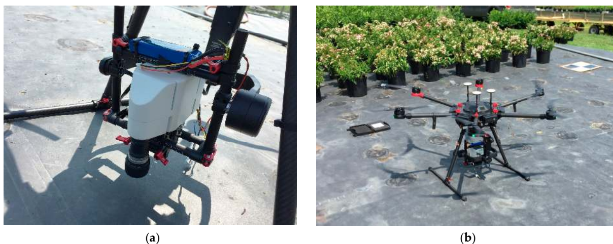
Figure 8. (a) Hyperspectral camera used for data collection, and (b) camera mounted on the Matrice 600 Pro drone for aerial imaging.
