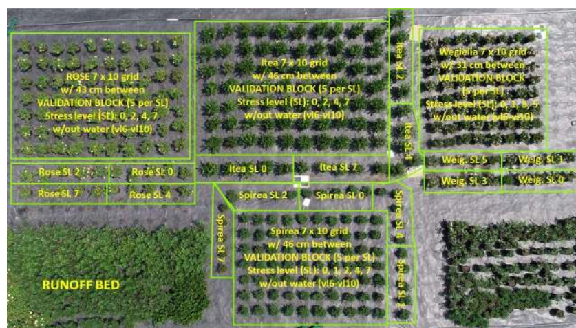
Figure 7. The experimental layout shows the arrangement of rose, itea, spirea, and weigela plants in 7 \times 10 grids, with designated validation plants and stress levels indicated for each taxon.
