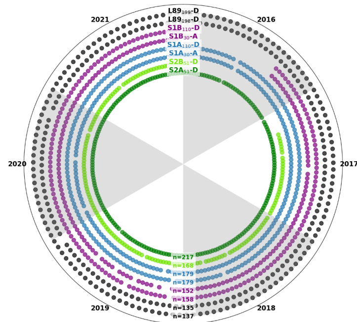
Figure 3. Chronogram of satellite acquisitions from 2016 to 2021. Sentinel-1A and 1B acquisitions are separated according to their orbit number (110 or 30) and direction (ascending: A or descending: D) (S1A 110-D , S1A 30-A , S1B 110-D , and S1B 30-A ) as Landsat-8 (L8 199-D and L8 198-D ) and Sentinel-2 data (S2A 051-D and S2B 051-D ).
