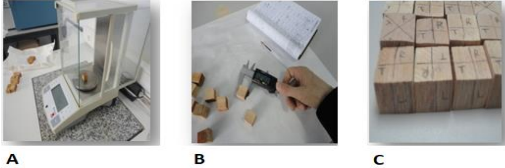
Fig. 6. The measurement of the mass of the test pieces by using a precision balance (photo A) and the dimensions following the three RTL directions (photos B and C) using a precision digital caliper
