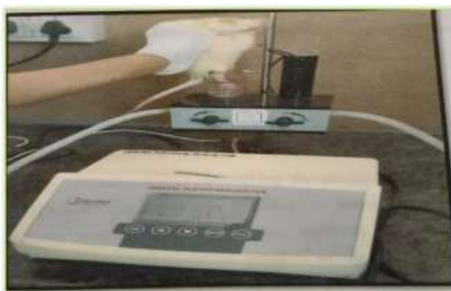
Figure 3: Measurement of Paw volume with the use of Plethysmometer
