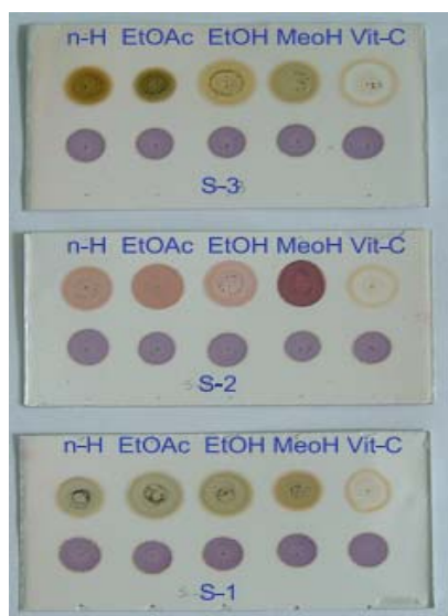
Fig.2 Scan of dot-blot test of a TLC Plate spotted with 0.4mM DPPH solution in methanol after fractions of each extract (n-hexane fraction, ethyl acetate fraction, ethanol fraction, methanol fraction) and L-ascorbic acid (vitamin-C) was applied. Control is 0.4mM DPPH solution in methanol.
