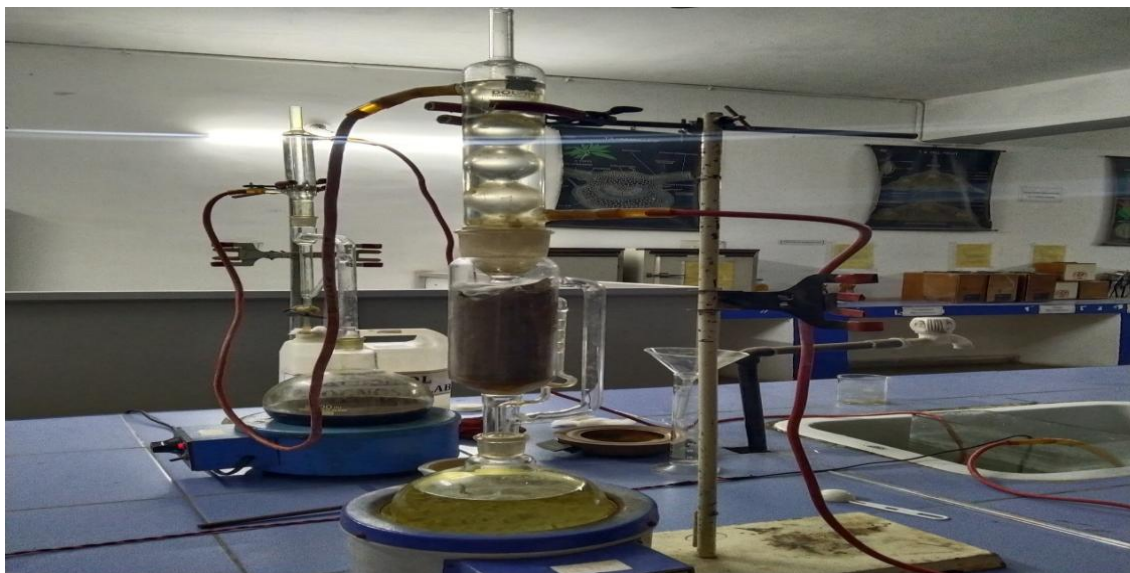
Figure 2.2.: Complete setup of Soxhlet apparatus carrying out the extraction of Cordia dichotoma leaves
