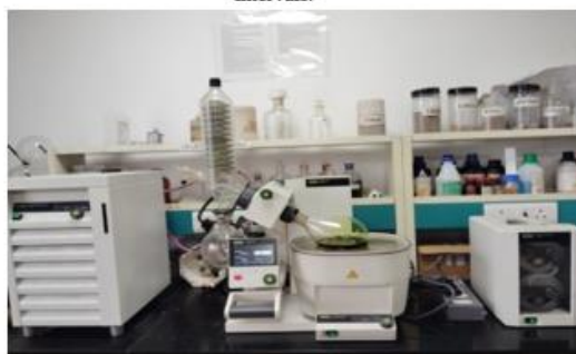
Figure 6. Final extract of Salix alba L. in the China Dish placed on REMI Water Bath for removal of any additional solvent to get a clarified extract.
