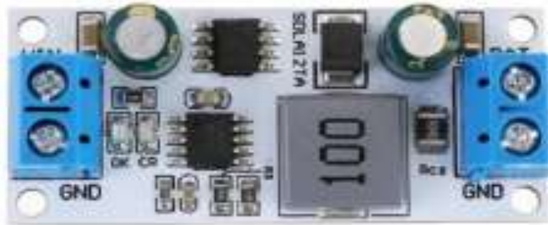
Figure 14:- Battery charger module.
