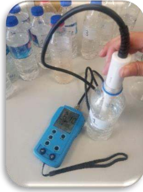
Picture 1. EC measurements of water samples
