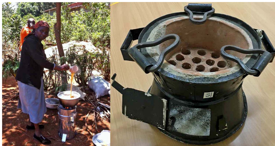
Figure 1. Galvanised steel gasifier cooking stove and Kenya Ceramic Jiko (KCJ) (Credit: M Njenga).
