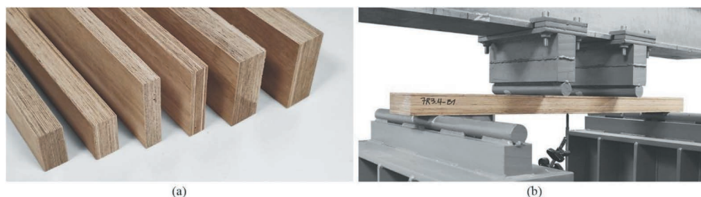
Figure 4. (a) LVL made of Eucalyptus globulus L; (b) flatwise bending test of a eucalyptus LVL specimen.
