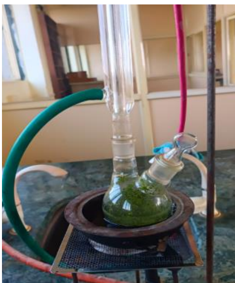
Fig. Extraction method (Reflux)
