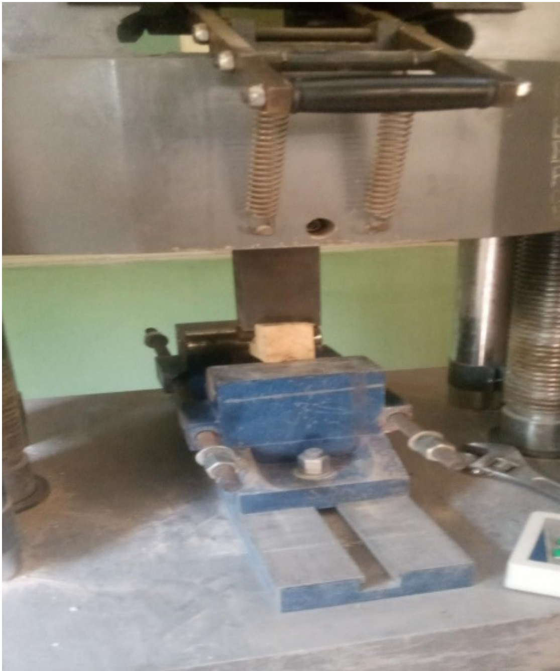
Fig. 3: Universal Testing Machine showing Shear Strength Test
