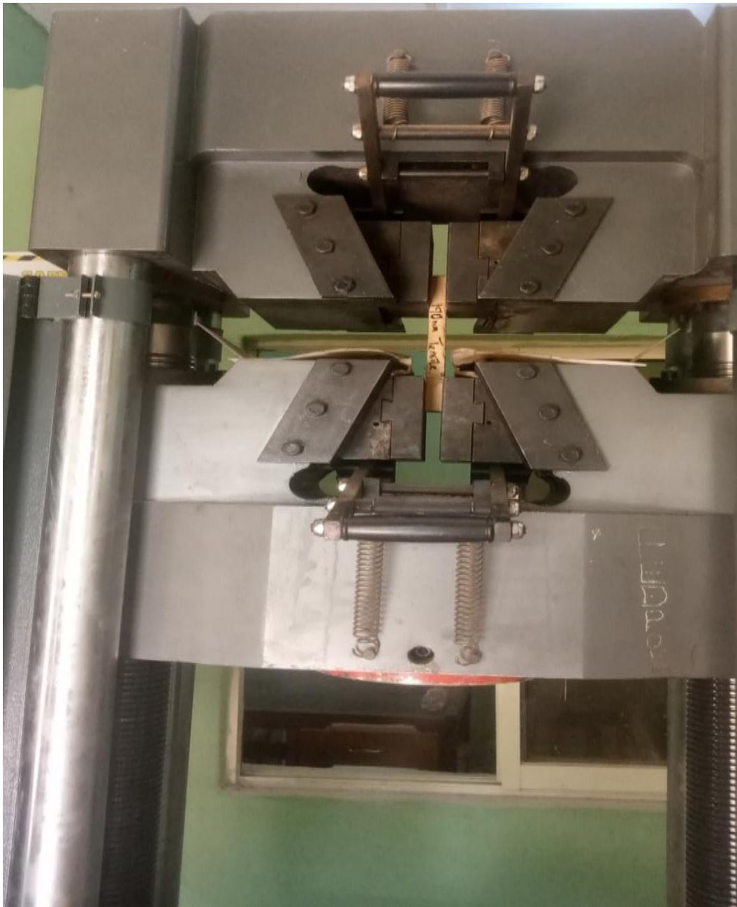
Fig. 2: Universal Testing Machine showing Tensile Strength Test
