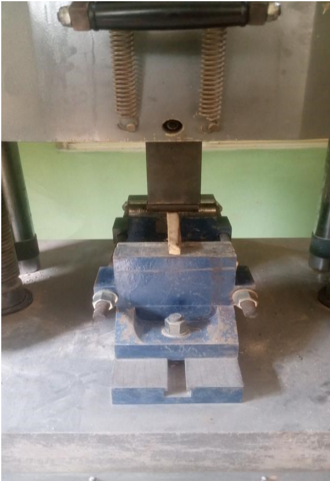
Fig. 4: Universal Testing Machine showing Static Bending Strength Test
