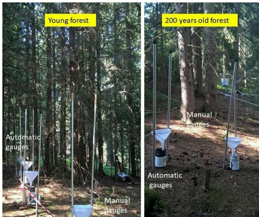
Figure 2. Measurement equipment (automated and manual gauges) put at soil level in both young and mature forests
