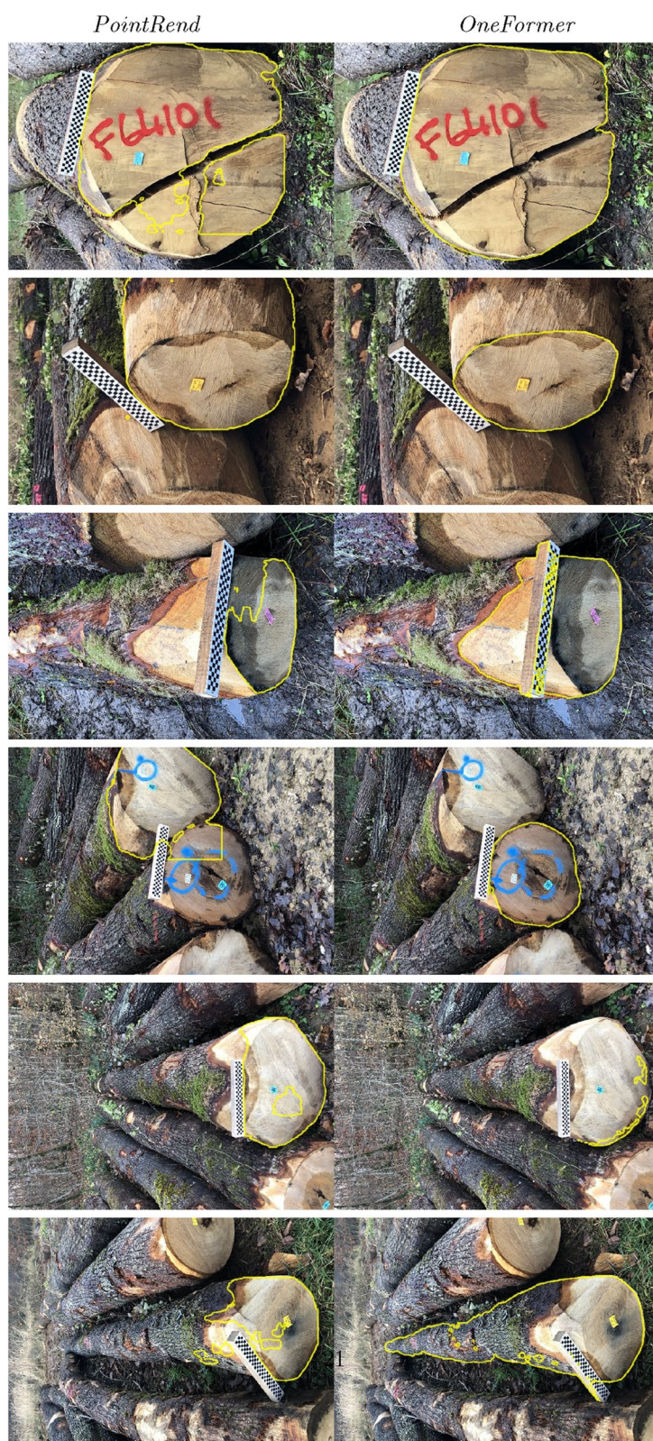
Fig. 7 Examples of the largest divergences obtained (in segmented surface area, for the first three rows, or in centre of gravity position, for the last three rows) for automatic segmentations performed using the PointRend (on the left) and OneFormer (on the right) architectures
