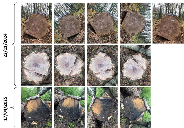
Fig. 1 Example of images collected for one log from case study #1. On the first date, five photos were taken of the cross-section (including the last one with a label) (on the first row), as well as four photos of the stump (on the second row). On the second date, four photos of the cross-section were taken again (on the third row)
