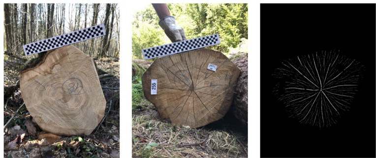
Fig. 8 Image taken at a first date on 17 February 2025 (on the left); image taken at a later date on 30 June 2025 showing drying cracks (in the middle); binary reference mask for marking drying cracks (on the right)
