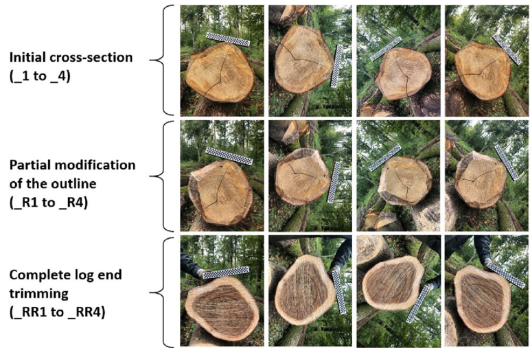
Fig. 3 Example of images collected for one log from case study #3. The initial cross-section is on the first row; the cross-section whose outline has been slightly modified is on the second row; the cross-section after complete log end trimming is on the third row
