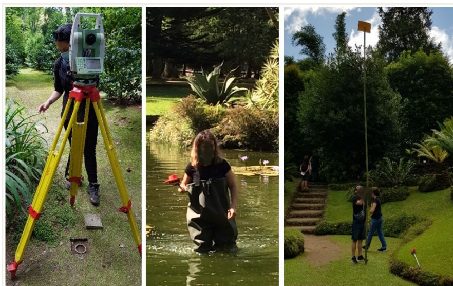
Fig. 3. Data acquisition with Total Station technique and at right an offset point with reflector elevation.
