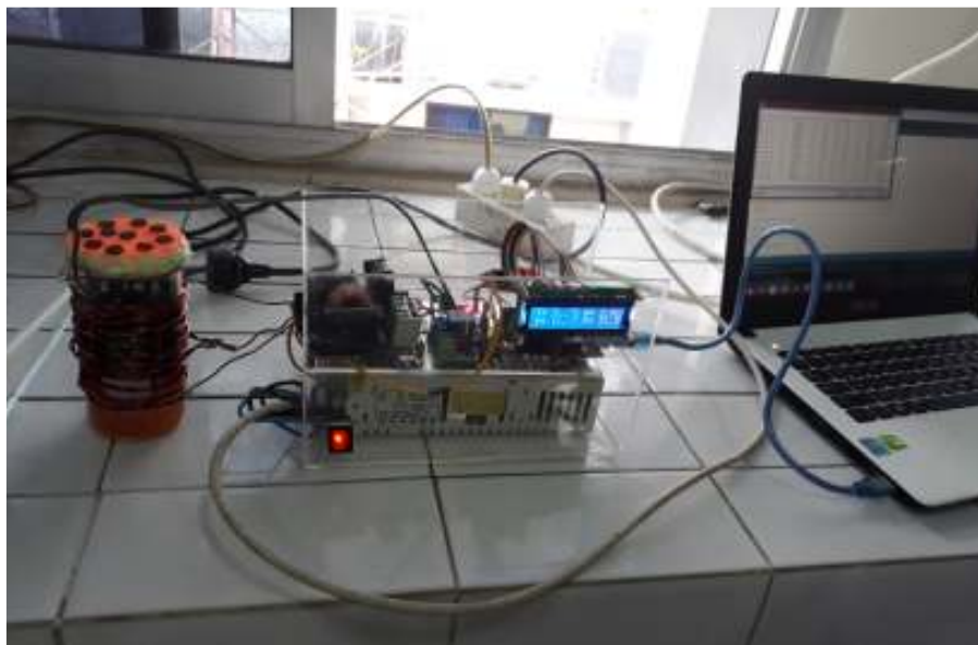
Figure 8. The esterification process using electromagnetic induction
