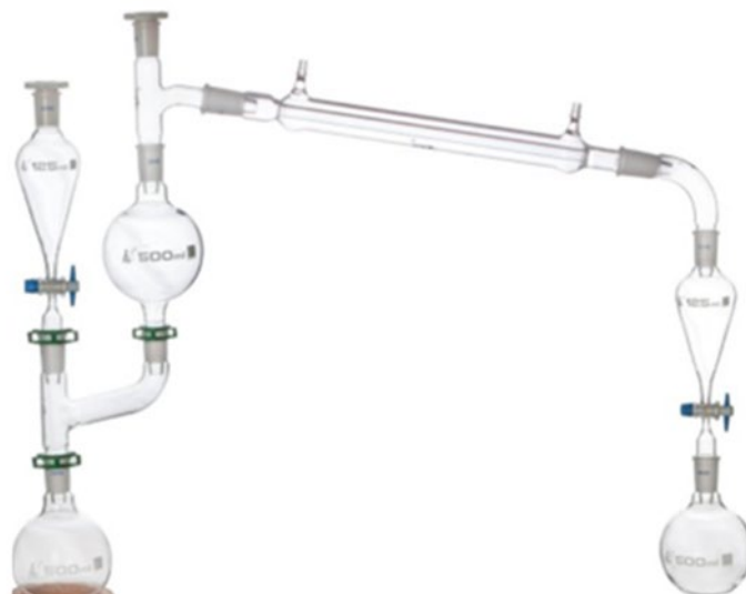
Figure 1. Steam Distillation Apparatus Used for Extraction Studies
