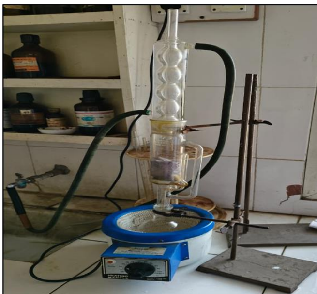
Figure no.4 Extraction of Jamun seed powder using Soxhlet Extractor
