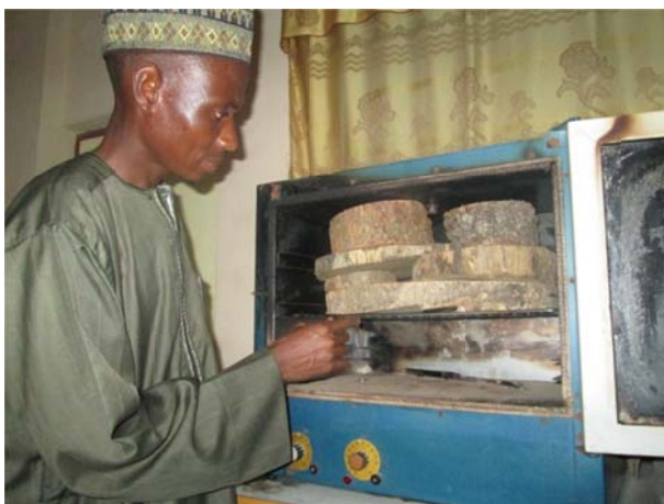
Fig. 7 Oven drying of aliquots
