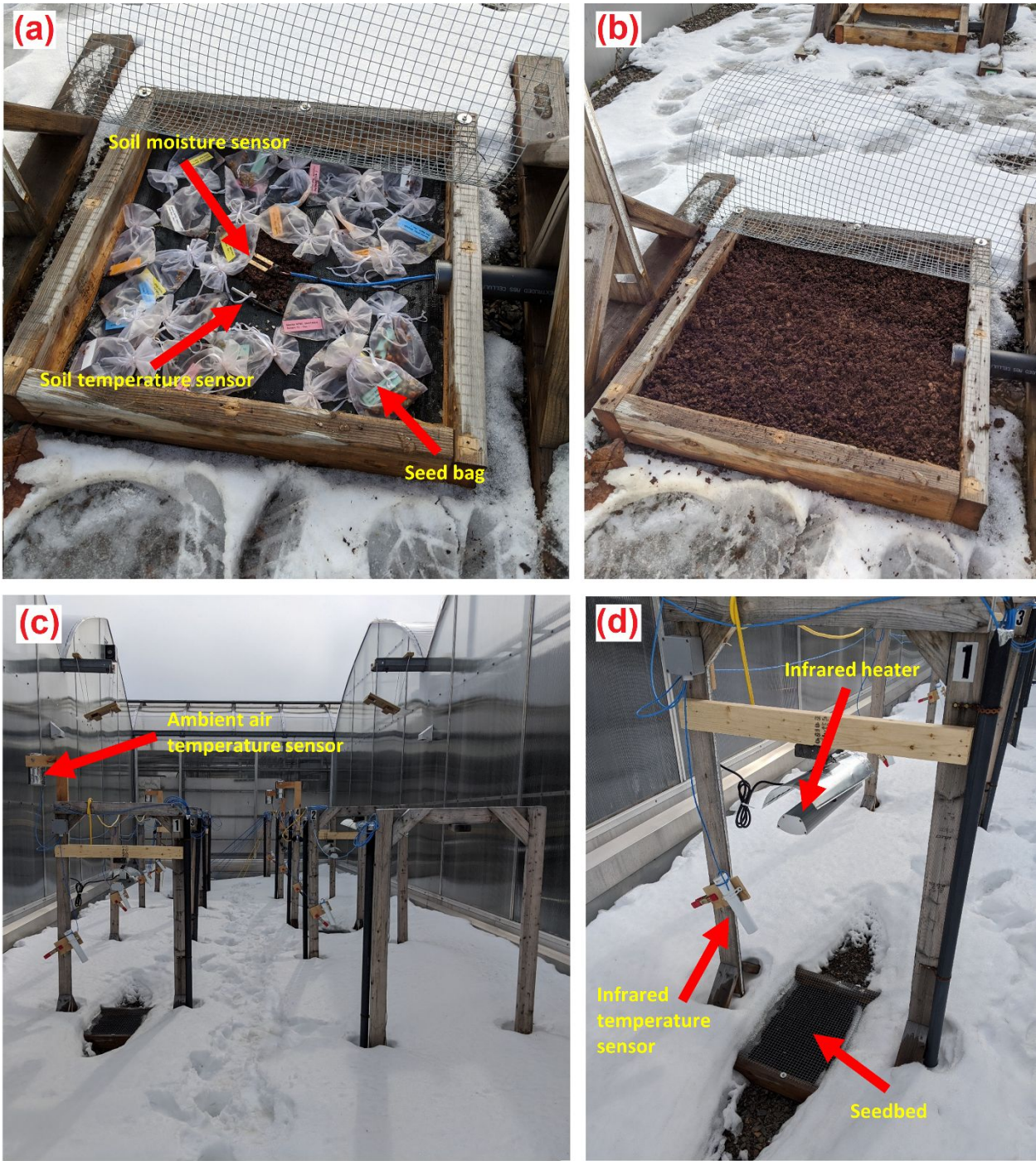
592 Figure 1. Seed plot layout and design: (a) arrangement of the 24 seed bags within one seedbed 593 and locations of the soil temperature and moisture sensors; (b) the seedbed after the seed bags 594 were covered with peat moss; (c) the entire site where the eight plots were set up in two rows of 595 four (the closest plot was not used) and the location of one of the ambient air temperature 596 sensors; and (d) location of the seedbed relative to the infrared heater and infrared temperature 597 sensor.
