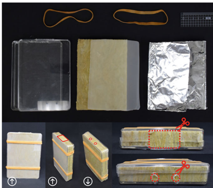
Fig. 1 Materials and structure of a rhizotron
