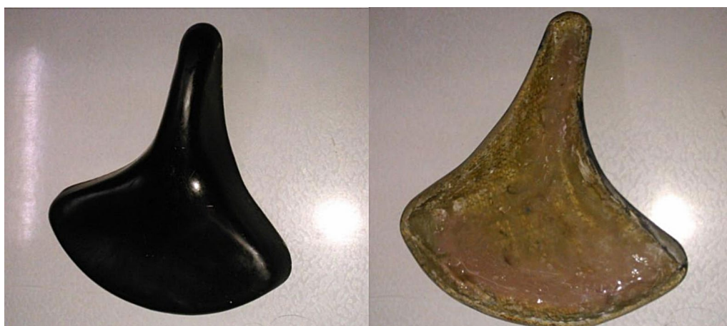
Fig. 9 Outer side view and Inner side view of cycle seat fabricated by AVFRVM polyester composite
