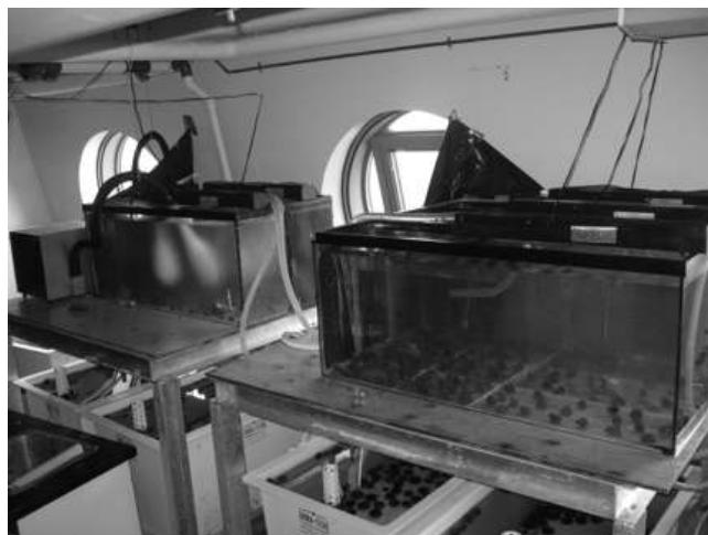
Figure 5. Experimental tank layout at the Ocean Sciences Centre at Logy Bay, NF. High-light right end of each tank is adjacent to large port-like window and has fluorescent lights overlying. Opposite, low-light ends of tanks shielded with opaque plastic sheet. Note cooling probes, coated with ice, placed in 2 and 4 °C tanks on left. Three light segments (left to right: low light, ll; mid-light, ml; high light, hl) with their emplaced specimens can be seen in right tank.
