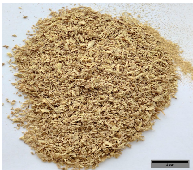
Fig. 2 Wood particles extracted by drill from the disc of Robinia pseudoacacia L. before grinding
