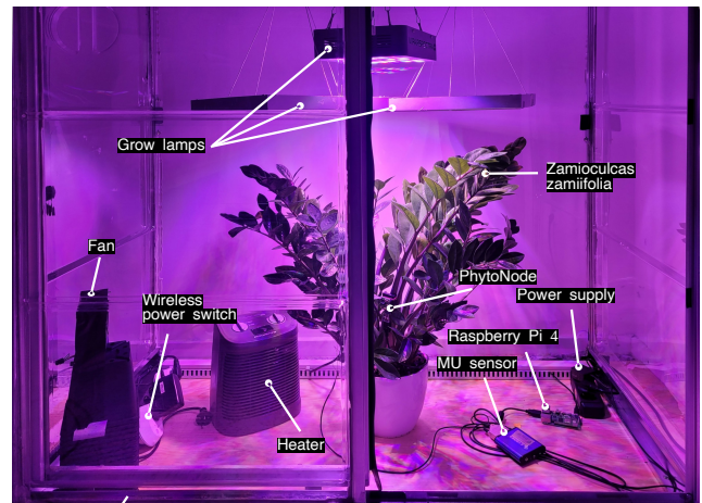
Figure 4: The full experiment setup. It includes the PhytoNode attached to Zamioculcas zamiifolia , grow lamps, a fan, a heater, a wireless power switch, a Raspberry Pi 4, a CYBRES MU sensor, and a power supply.
