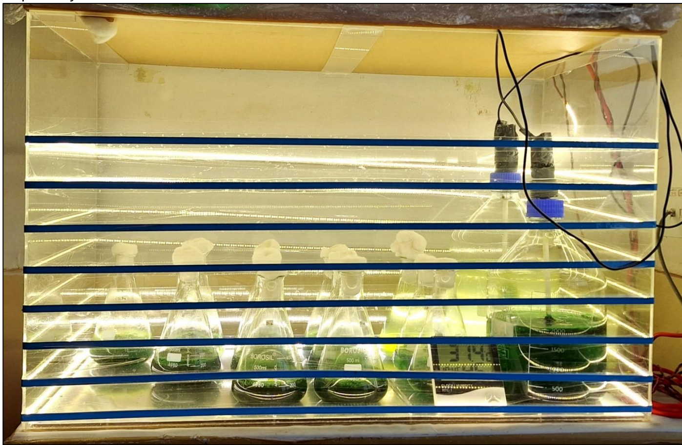
Figure 1. Lab-scale photobioreactor setup for the phototrophic cultivation of S. subsalsa and C. pyrenoidosa under controlled light and temperature conditions.
