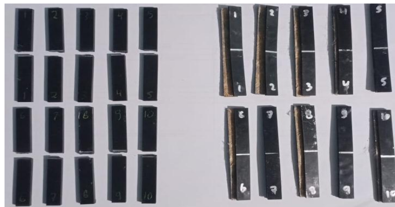
Figure 2. Fracture of impact test specimens for variation 1 (rPP 100%) (left) and variation 2 (rPP 98%:2% by weight biduri fiber; KOH 0%) (right).
