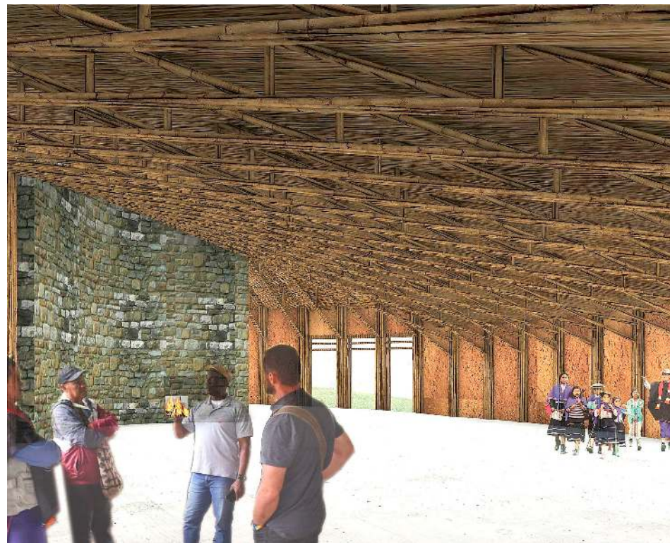
Figure 19. Interior rendering of volume with a roof with the geometry of a freeform surface with strategic windows. Drawings by students of the course “Digital, optimal and smart structures”, directed by authors of this paper.
