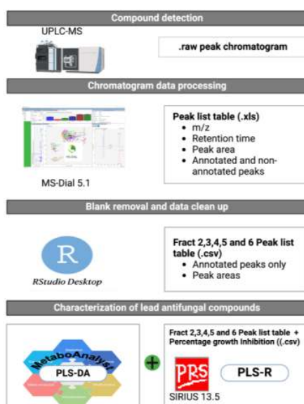
Figure S2 Workflow for the metabolomic identification and characterization of lead antifungal compounds. All samples (NCE, chemical extracts, and fractions) were separated and analyzed using UHPLC-MS. The resulting raw chromatograms were processed in MS-DIAL to extract and quantify features, followed by a tentative annotation. Lead antifungal compounds were identified by integrating chemometric analysis (PLS-DA, using MetaboAnalyst) with biochemometric modeling (PLS-R, using SIRIUS 13.5).
