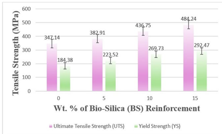
Figure 6: The IGT and IGT/BS nanocomposites ultimate tensile and yield strengths.
