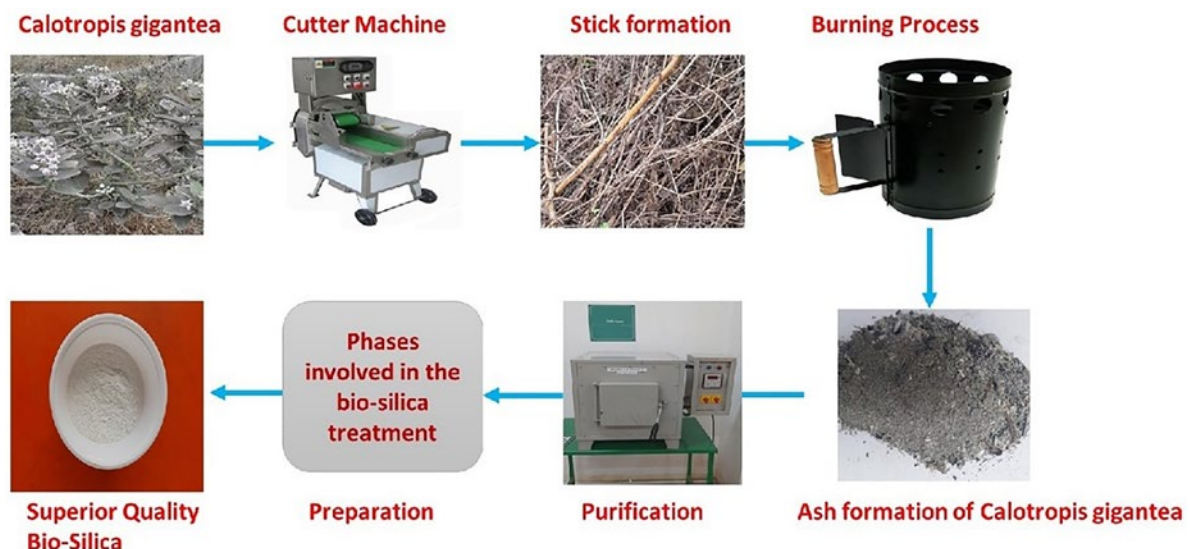
Figure 1: Synthesis of bio-silica nano reinforcing particles derived from Calotropis .
