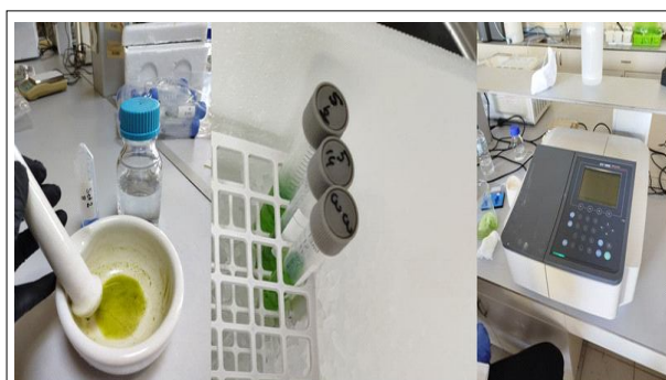
The workflow includes (i) Grinding fresh leaf tissue, (ii) Transferring samples into pre-labeled cooled tubes for pigment extraction and (iii) Spectrophotometric measurement of absorbance values for chlorophyll a, chlorophyll b and total carotenoids.
