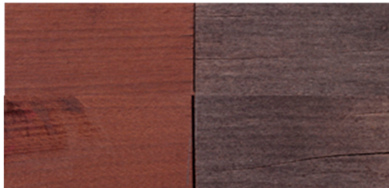
Figure 4. The visual appearance of thermally modified beech wood specimens (210 °C, 2 h) before ( left ) and after weathering ( right ).
