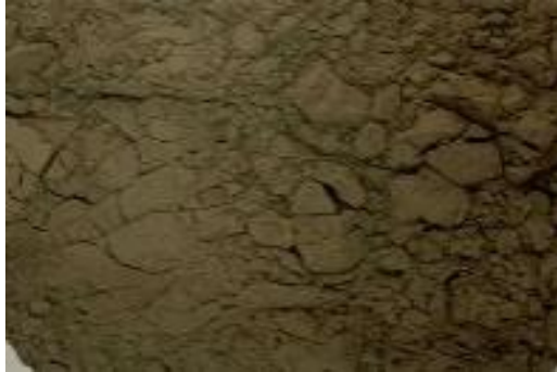
Figure 1. Appearance of Fly Ash
