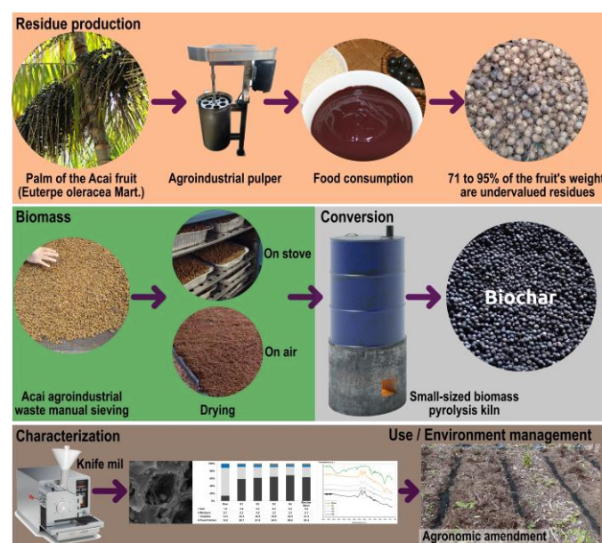
Figure 1. Generation of residues from the acai agro-industry; pre-treatment of biomass for pyrolysis and biochar production; post-treatment involving grinding and characterisation of the biochar; its use in agronomic experiments.
