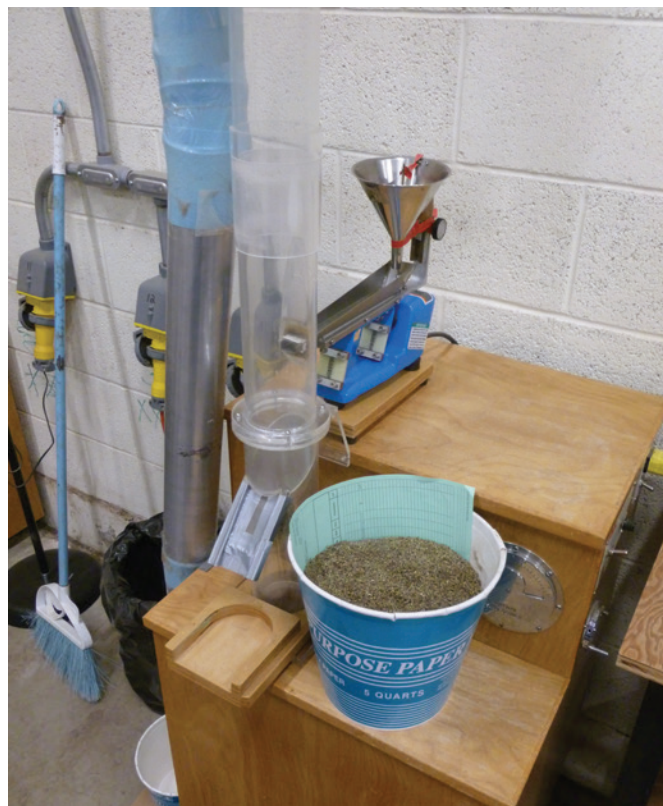
Brushed (Westrup LA-H brush machine) yellow Indian paintbrush seed-bearing material ready to be passed through an air column separator (background) to separate chaff from seed.
