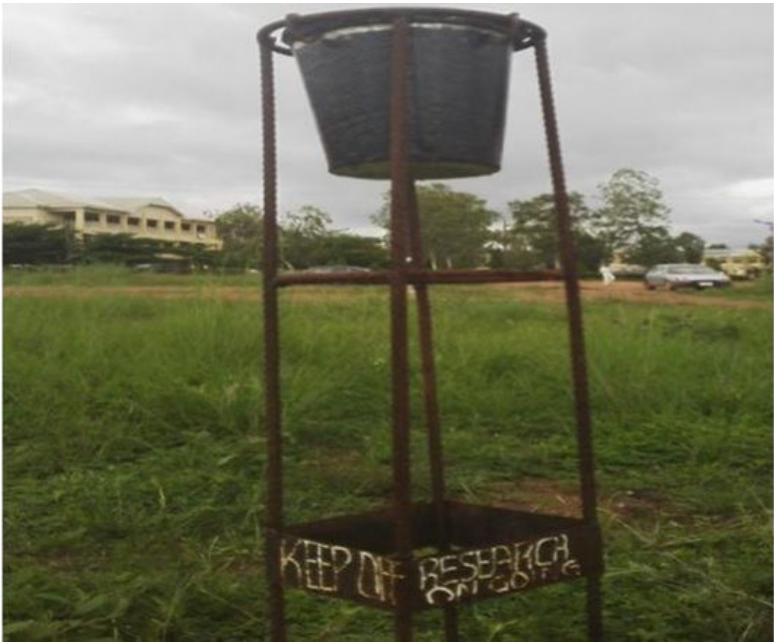
Figure 2 A mounted pollen sampler at the sampling station in Ebonyi State University, Ebonyi State, Nigeria.
